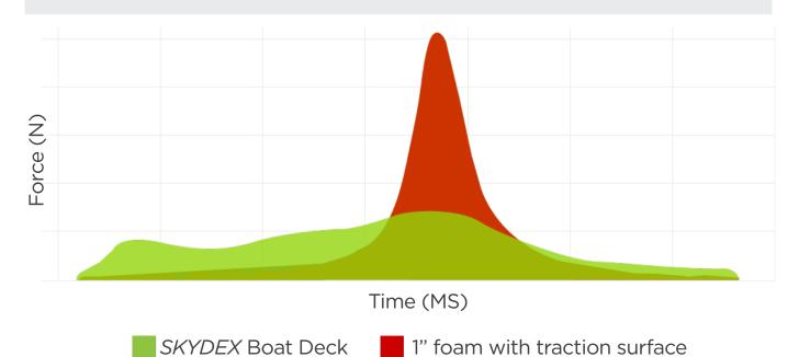
*SKYDEX* Boat Decking is designed to mitigate the force of an impact by absorbing energy over a longer period of time compared to foam products
